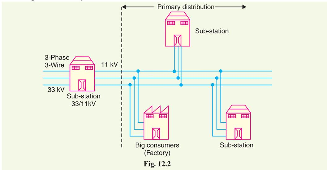
Fig. 12.2 shows a typical primary distribution system. Electric power from the generating station is transmitted at high voltage to the substation located in or near the city. At this substation, voltage is stepped down to 11 kV with the help of step-down transformer. Power is supplied to various substations for distribution or to big consumers at this voltage. This forms the high voltage distribution or primary distribution.
