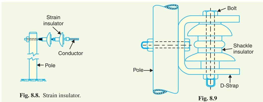
Fig. 8.8. Strain insulator.
