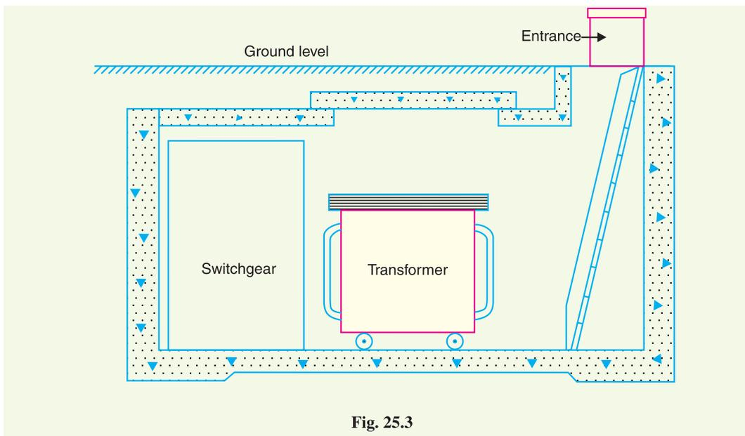
The design of underground sub-station requires more careful consideration than other types of sub-stations. While laying out an underground sub-station, the following points must be kept in view:
