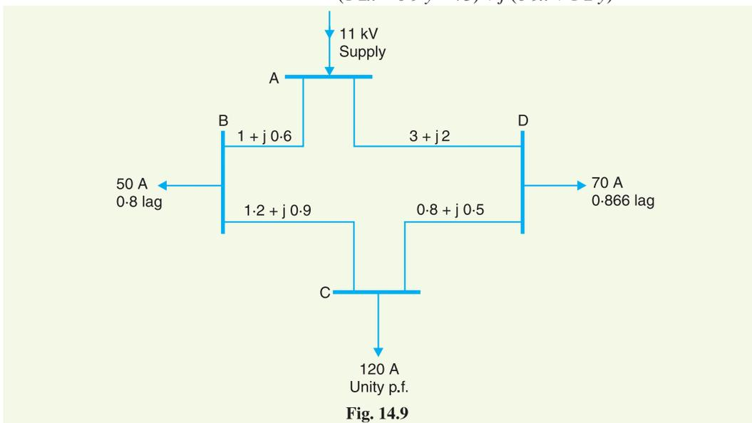
$$\begin{aligned}\text{Drop in section } CD &= \vec{I}_{CD} \vec{Z}_{CD} \\ &= [(x - 160) + j(y + 30)] [(0.8 + j0.5)] \\ &= (0.8x - 0.5y - 143) + j(0.5x + 0.8y - 56)\end{aligned}$$
