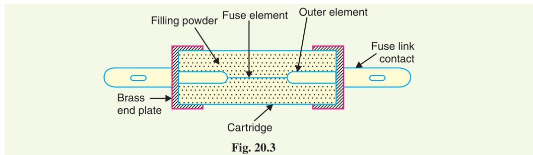
Under normal load conditions, the fuse element is at a temperature below its melting point.
