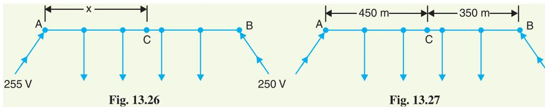
**Example 13.16.** A 800 metres 2-wire d.c. distributor AB fed from both ends is uniformly loaded at the rate of 1.25 A/metre run. Calculate the voltage at the feeding points A and B if the minimum potential of 220 V occurs at point C at a distance of 450 metres from the end A. Resistance of each conductor is 0.05  $\Omega$ /km.
