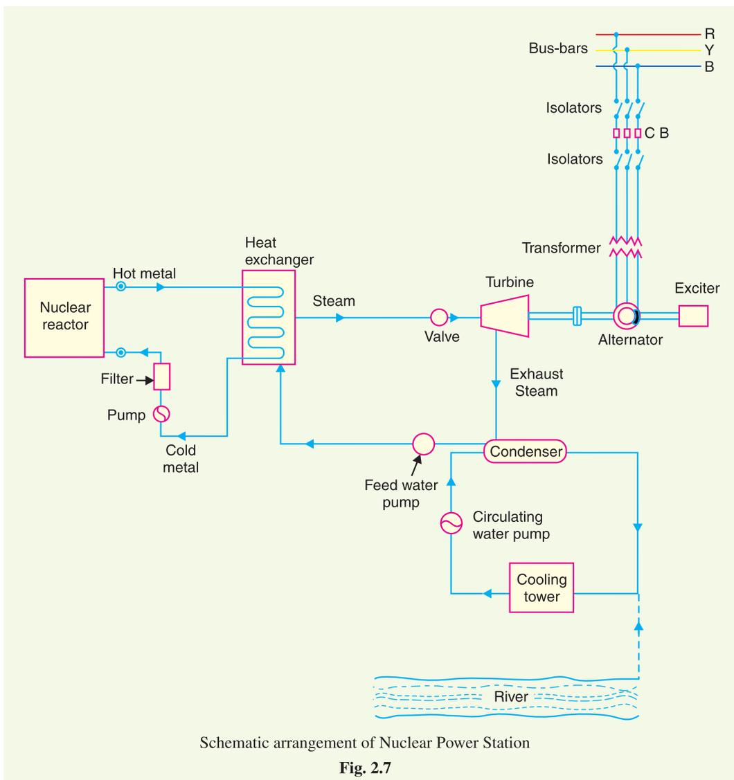
(i) **Nuclear reactor.** It is an apparatus in which nuclear fuel ( $U^{235}$ ) is subjected to nuclear fission. It controls the *chain reaction*\* that starts once the fission is done. If the chain reaction is not controlled, the result will be an explosion due to the fast increase in the energy released.
