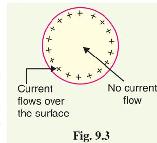
\* For a direct current, inductance is zero and hence the current distributes uniformly over the entire X-section of the conductor.
