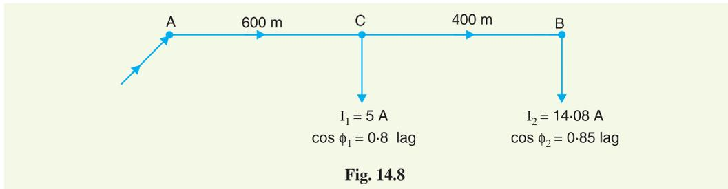
$$\text{Phase voltage at point B, } V_B = 400/\sqrt{3} = 231 \text{ V}$$
