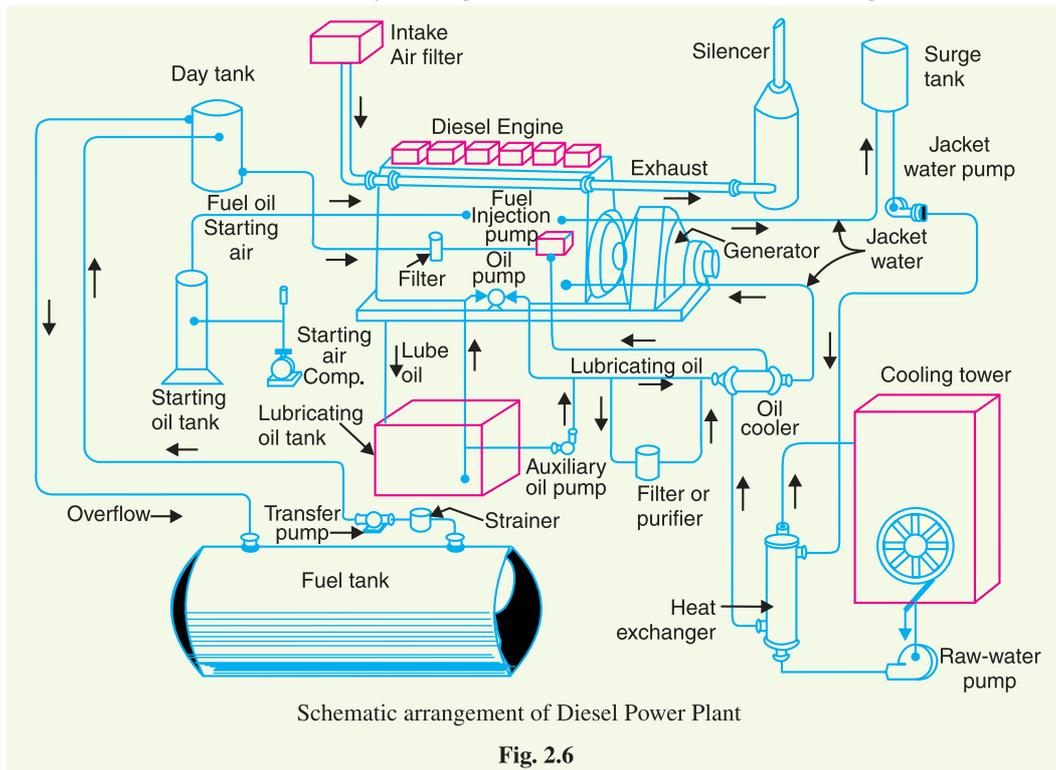
(v) **Lubricating system.** This system minimises the wear of rubbing surfaces of the engine. It comprises of lubricating oil tank, pump, filter and oil cooler. The lubricating oil is drawn from the lubricating oil tank by the pump and is passed through filters to remove impurities. The clean lubricating oil is delivered to the points which require lubrication. The oil coolers incorporated in the system keep the temperature of the oil low.
