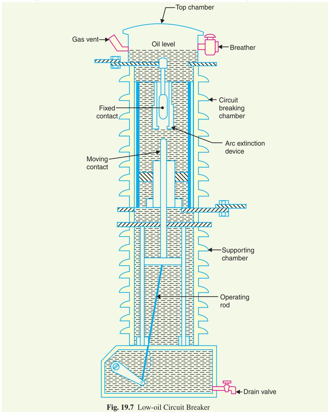
Fig. 19.7 Low-oil Circuit Breaker
