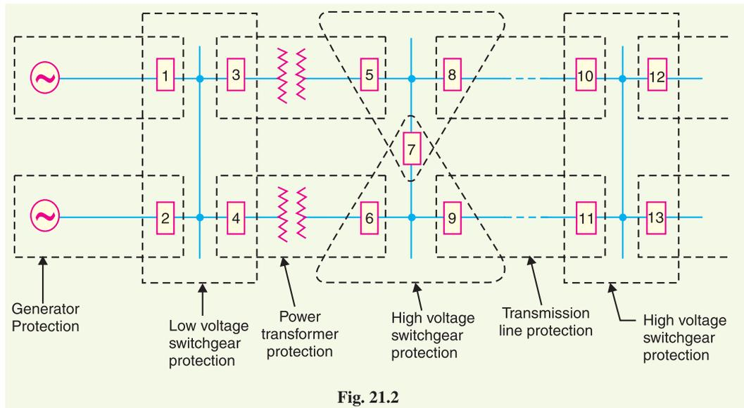
In order to provide selectivity to the system, it is a usual practice to divide the entire system into several protection zones. When a fault occurs in a given zone, then only the circuit breakers within that zone will be opened. This will isolate only the faulty circuit or apparatus, leaving the healthy circuits intact. The system can be divided into the following protection zones :
