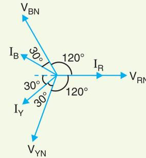
**Solution.** Fig. 14.17 shows the circuit diagram whereas Fig. 14.18 shows its phasor diagram. The current  $I_R$  is in phase with  $V_{RN}$ , current  $I_Y$  lags behind its phase voltage  $V_{YN}$  by  $\cos^{-1} 0.866 = 30^\circ$  and the current  $I_B$  leads its phase voltage  $V_{BN}$  by  $\cos^{-1} 0.866 = 30^\circ$ .
