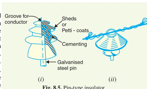
Fig. 8.5. Pin-type insulator
