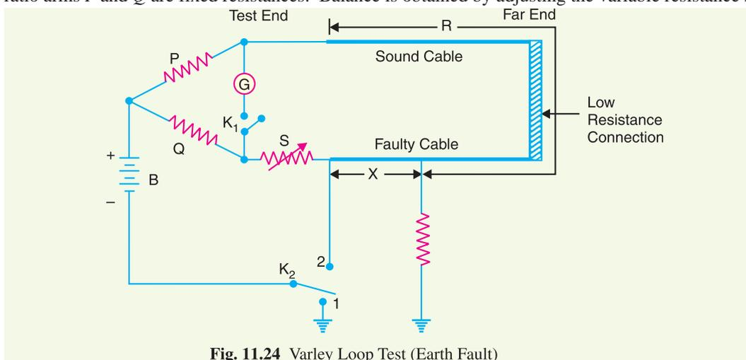
connected to the test end of the faulty cable. The connection diagrams for locating the earth fault and short-circuit fault by Varley loop test are shown in Figs. 11.24 and 11.25 respectively.
