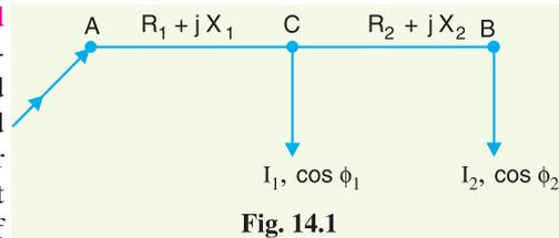
$$\text{Impedance of section } AC, \quad \overline{Z}_{AC} = R_1 + j X_1$$
