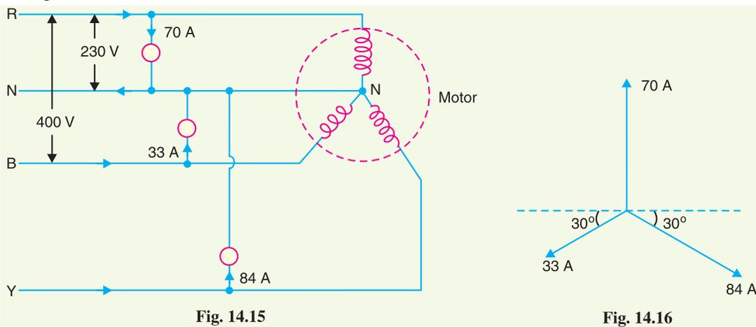
$$\begin{aligned} \text{Resultant H-component} &= 84 \cos 30^\circ - 33 \cos 30^\circ = 44.17 \text{ A} \\ \text{Resultant V-component} &= 70 - 33 \cos 60^\circ - 84 \cos 60^\circ = 11.5 \text{ A} \\ \therefore \text{ Neutral current, } I_N &= \sqrt{(44.17)^2 + (11.5)^2} = \mathbf{45.64 \text{ A}} \end{aligned}$$
