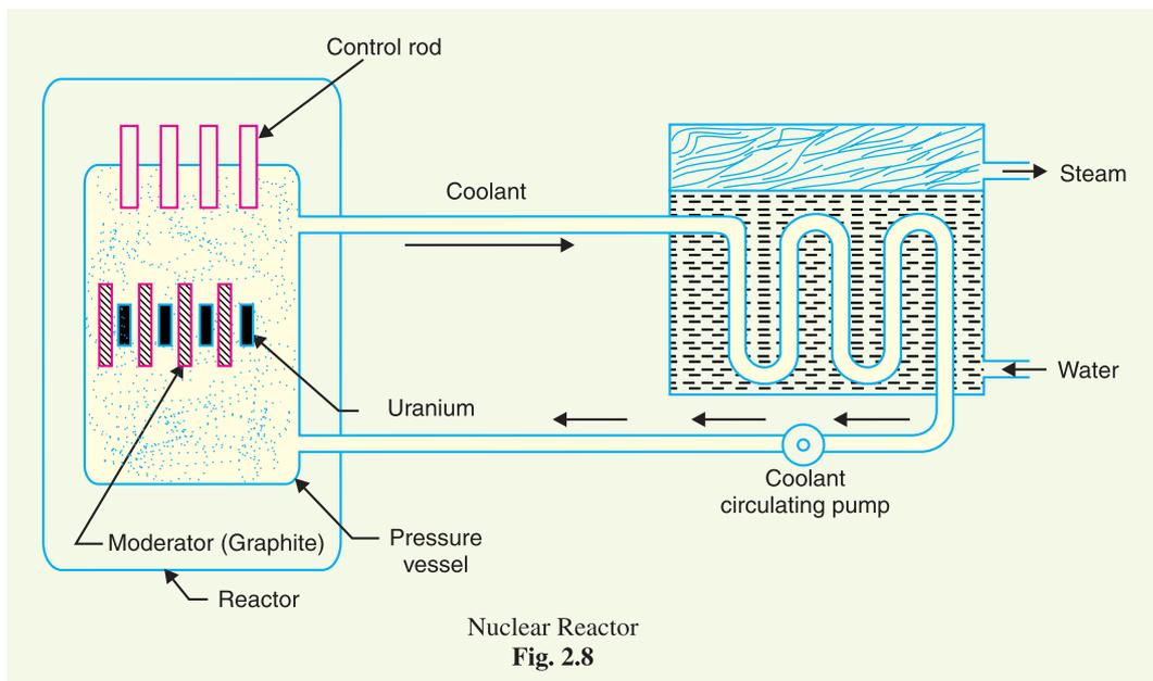
(ii) **Heat exchanger.** The coolant gives up heat to the heat exchanger which is utilised in raising the steam. After giving up heat, the coolant is again fed to the reactor.
