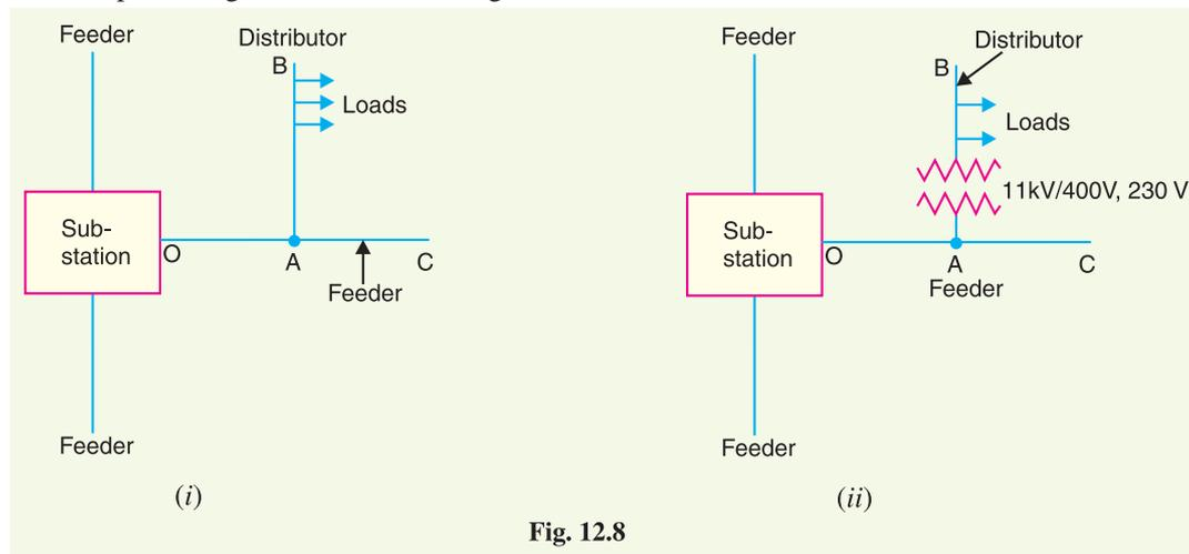
This is the simplest distribution circuit and has the lowest initial cost. However, it suffers from the following drawbacks :
