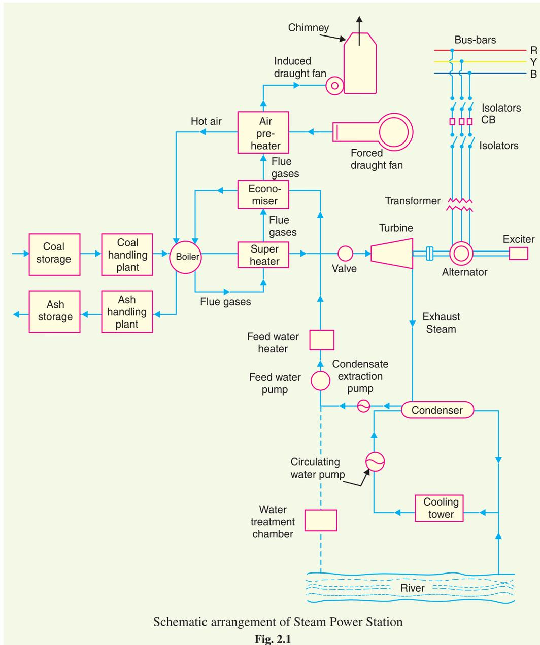
excess air. The pulverised coal is fed to the boiler by belt conveyors. The coal is burnt in the boiler and the ash produced after the complete combustion of coal is removed to the ash handling plant and then delivered to the ash storage plant for disposal. The removal of the ash from the boiler furnace is necessary for proper burning of coal.
