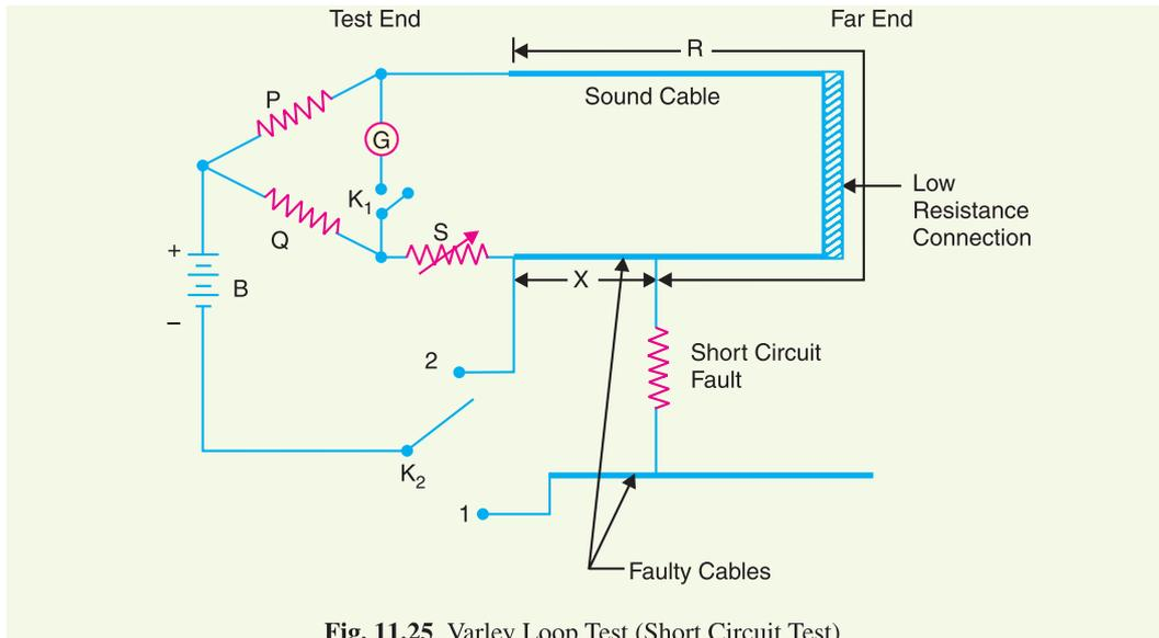
**Fig. 11.25** Varley Loop Test (Short Circuit Test)
