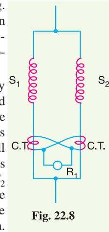
**Example 22.1.** A star-connected, 3-phase, 10-MVA, 6.6 kV alternator has a per phase reactance of 10%. It is protected by Merz-Price circulating-current principle which is set to operate for fault currents not less than 175 A. Calculate the value of earthing resistance to be provided in order to ensure that only 10% of the alternator winding remains unprotected.
