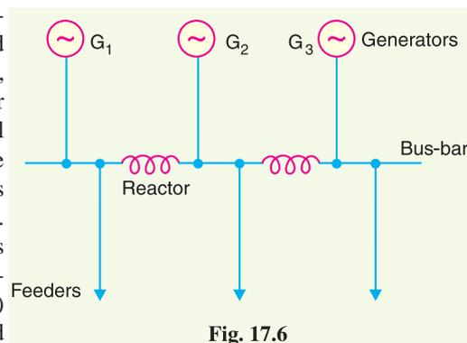
from other generators is small due to the presence of reactors. Therefore, only that section of bus-bar is affected to which the feeder is connected, the other sections being able to continue in normal operation.
