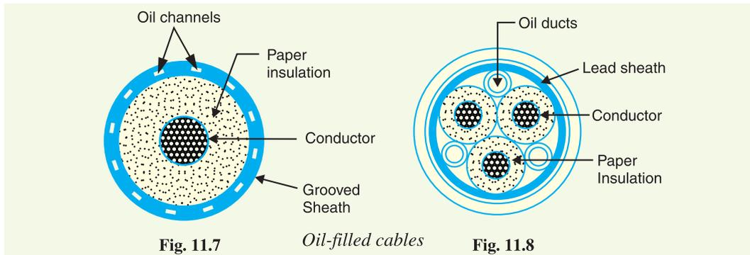
The oil-filled cables have three principal advantages. Firstly, formation of voids and ionisation are avoided. Secondly, allowable temperature range and dielectric strength are increased. Thirdly, if there is leakage, the defect in the lead sheath is at once indicated and the possibility of earth faults is decreased. However, their major disadvantages are the high initial cost and complicated system of laying.
