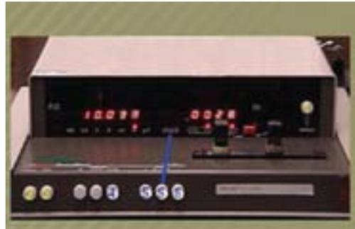
Capacitance Measurement using bridge
