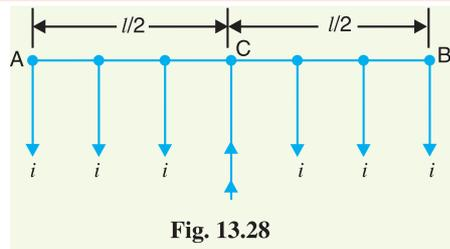
$$\begin{aligned} \therefore \text{Max. voltage drop} &= \text{Voltage drop in half distributor} \\ &= \frac{1}{2} \left( \frac{il}{2} \right) \left( \frac{rl}{2} \right) = \frac{1}{8} (il)(rl) \\ &= \frac{1}{8} IR \end{aligned}$$
