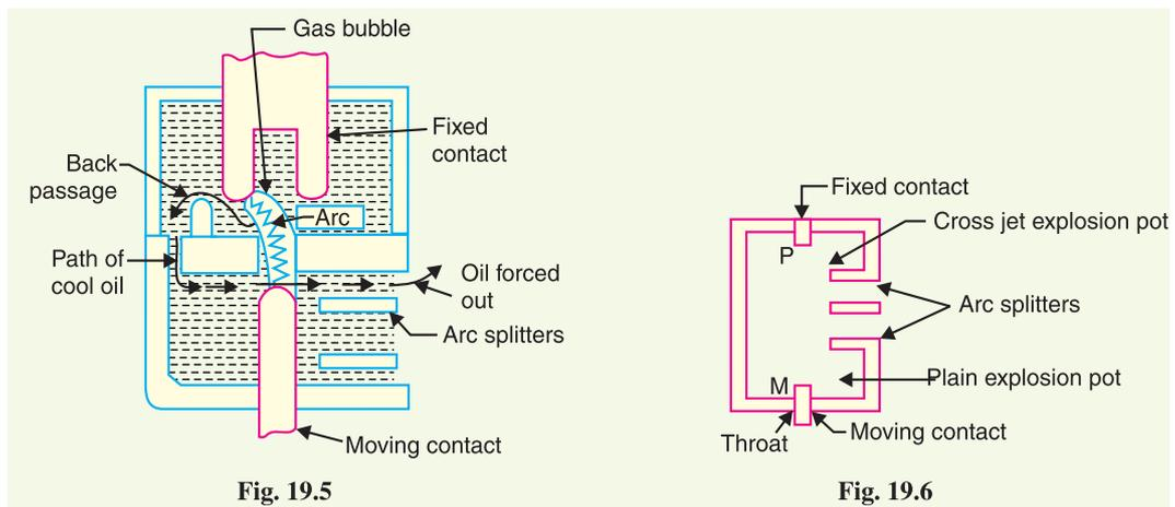
The cross-jet explosion pot is quite efficient for interrupting heavy fault currents. However, for low fault currents, the gas pressure is †small and consequently the pot does not give a satisfactory operation.
