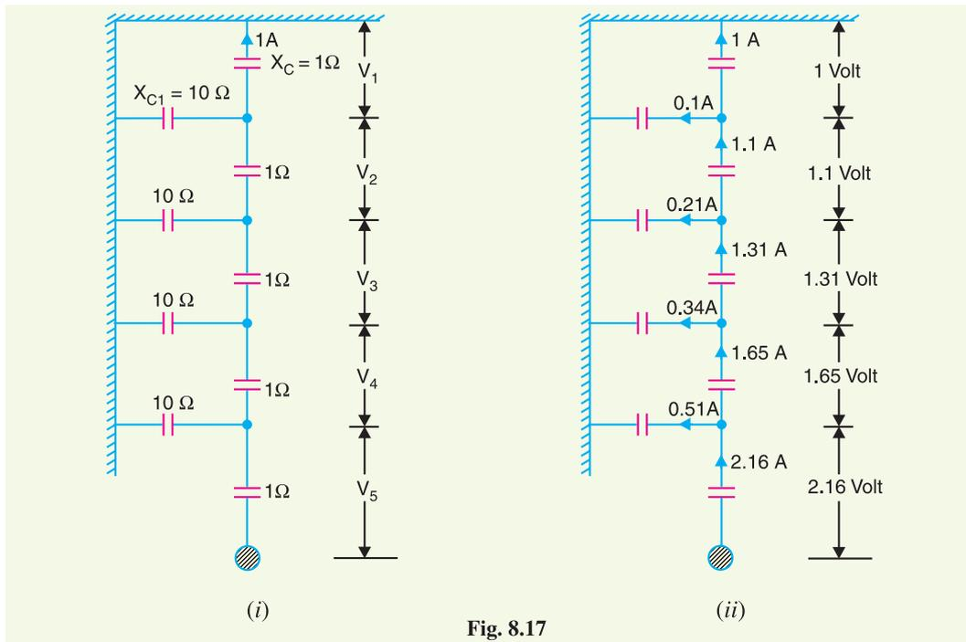
The value obtained for  $V = 1 + 1.1 + 1.31 + 1.65 + 2.16 = 7.22$  volts and starting from top, the percentage of  $V$  (i.e., 7.22 volts) across various units are :
