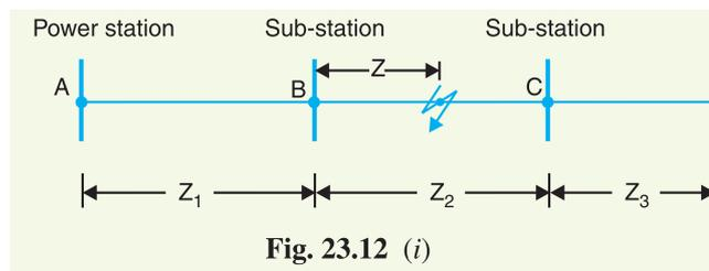
portion shown, only relay at  $B$  will operate. Similarly, if a fault occurs within section  $AB$ , then only relay at  $A$  will operate. In this manner, instantaneous protection can be obtained for all conditions of operation.
