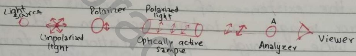
In the figure, unpolarized light passes through a filter so that only waves that oscillate in a certain direction can pass through. When these waves interact with an optically active material, they are rotated either clockwise or anticlockwise, depending on the enantiomer. In the case of the image above, the light is rotated clockwise so the substance is dextrorotatory enantiomer.
