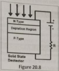
circuit. The combined thickness of N-type and gold layer absorbs so less energy of the incident particle that the junction may be assumed to be situated at the front surface as shown in fig 20.8.
