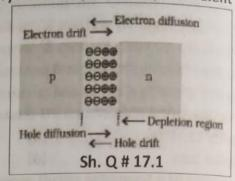
negative charge appears in P-region and vice versa. The electrons in P-region and holes in N-region stops further diffusion of electrons from N-side and holes from Pside respectively thus maintaining separation of charge carriers. This region of separation between charge carriers is free of mobile charges and it is called depletion region.
