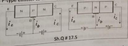
holes are received through reverse biased, collector-base configuration at the collector to form collector current. Hence total emitter current is distributed into two parts namely base current and collector current. Mathematical equation for current representation in PNP is same as eq (1) for NPN transistor. It may be noted that in P-type conductivity, the valence electrons move from one covalent bond to another unlike the N-type where current conduction is by free electrons.
