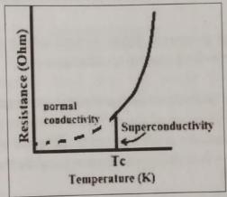
approaches smaller values of resistance till it becomes zero at Tc. The dashed curve also shows resistance of ordinary material that is not superconductor. Magnetic resonance imaging (MRI) and magnetic levitation trains are some of the applications of superconductors.
