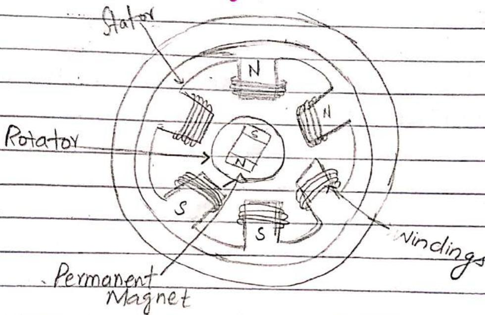
→ stator : A group of electromagnets arranged around cylinder with poles facing towards stator poles.
