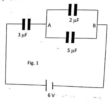
Let  $C_{eq}$  be the net capacitance of fig.2, then  $C_{eq} = \frac{C_1 C_{AB}}{C_1 + C_{AB}} = \frac{3 \times 7}{3 + 7} = \frac{21}{10} = 2.1 \, \mu F$
