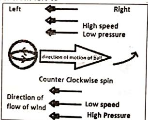
the pressure below the ball increases. Due to this un-even pressure the ball will tend to deflect from high pressure side towards low pressure side. Therefore the ball will move away from the observer.
