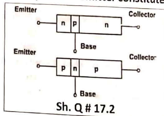
**(b)** Collector current is the current which is supplied to the load. The key role of the collector is to receive the charges from base to constitute collector current. Transistor must be configured in such a way that almost all the emitter current is received at the collector. For this purpose collector is made larger in size so that all the charges can be received at the collector as shown in the figure.
