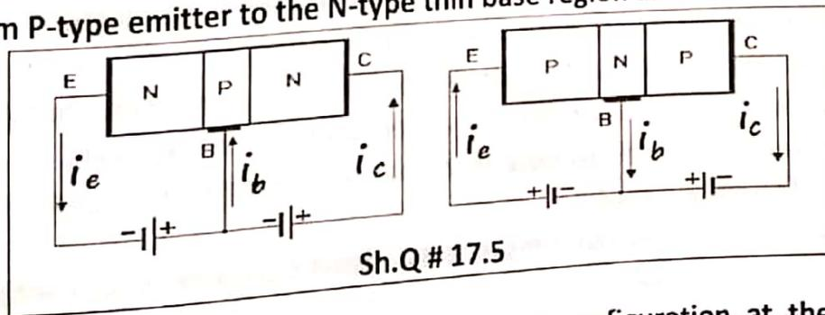
that in P-type conductivity, the valence electrons move from one covalent bond to another unlike the N-type where current conduction is by free electrons.
