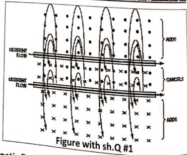
between the conductors while magnetic fields outside the conductors add up. Now by applying right hand rule it can be shown that force on first conductor is towards second and force on second conductor is towards first conductor. It means that both the conductors attract each other. This can be understood easily by the figure shown.
