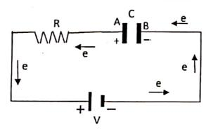
From the circuit,  $V = V_R + V_C \rightarrow (1)$ . Initially the charge on the capacitor is zero therefore,  $V_C = Q/C$ , will be zero and the whole voltage of the source will be available across resistor only. But gradually when the capacitor charges  $V_C$  will increase. As V (source voltage) remains constant therefore, according to eq.1  $V_R$  will decrease.
