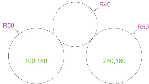
Fig. 2.15 Second example – Circle tool. The radius-40 circle tangential to the radius-50 circles
