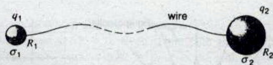
FIGURE 28-21. Two conducting spheres connected by a long thin wire.
