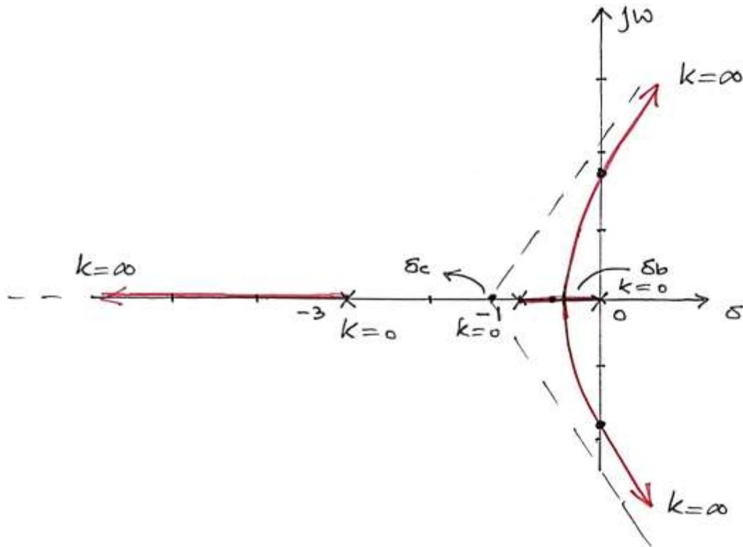
1. We can see that now the root locus is not a vertically straight line but it follows a curve and crosses the  $j\omega$ -axis. Thus adding a pure integrator will make the otherwise stable system to a system that may lead to instability if the operating point is not wisely selected.
