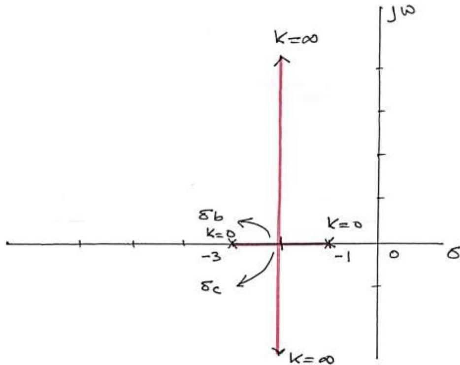
The root locus is a straight vertical line and therefore does not cross the  $j\omega$ -axis. Thus the system does not move into the unstable region (right-half plane) and is therefore always stable. Thus all the closed-loop poles lie in the left-half plane.
