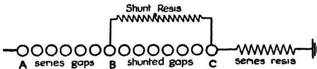
FIG. 141.—Diagram of 'low-equivalent' multiple-gap arrester.
