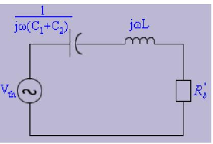
The equivalent circuit of a CCVT is shown in figure. The values of C1 and C2 are 0.0018  $\mu$ F and 0.0186  $\mu$ F respectively. Tuning inductor has an inductance of 497H and resistance of 4620  $\Omega$ . X<sub>m</sub> of the VT referred to 6.6 kV side is 1M $\Omega$ , core loss = 20 watts per phase, VA burden = 150VA per phase. Value of Cm for compensating the current drawn by Xm is equal to 3.183 nF.
