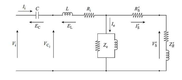
Resistance of the secondary circuit and the load impedance are represented by  $R_s$  and  $Z_B$ , respectively, whereas  $V_s$  and  $I_s$  represents the secondary voltage.
